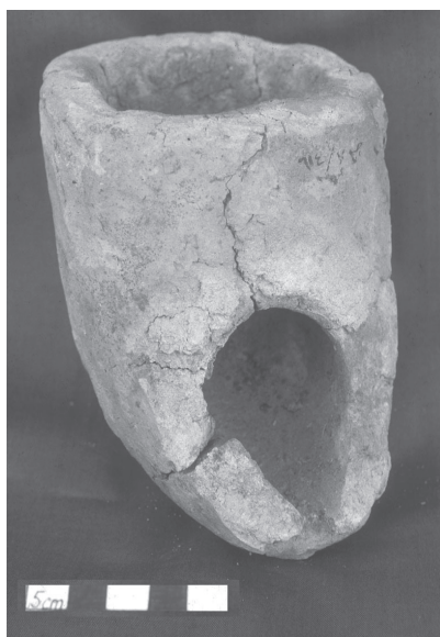
Fig. 5. Picture of Crucible 614/7 showing the white colouring at the front and stress fractures (Photo CJ Davey).
