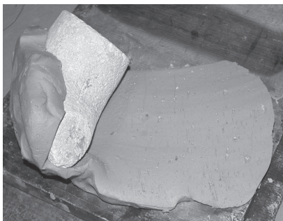
Fig. 7. Making a replica crucible over a horn-shaped pattern (Photo CJ Davey).
